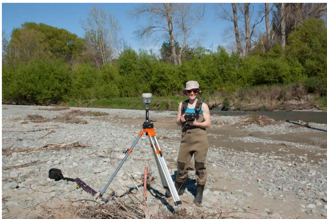
Surveying location of mini-piezometers. Photo credit: Peter Joynt
