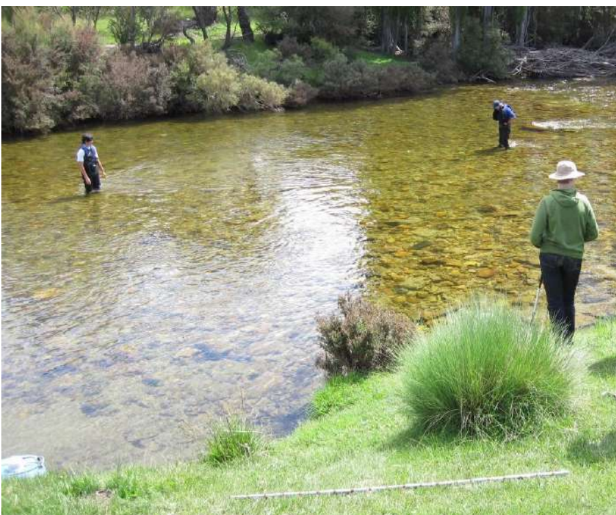
Undertaking surface velocity measurements at the gauging station
