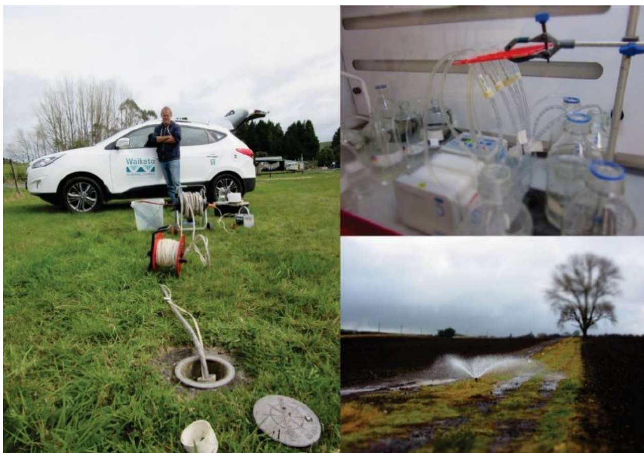
Figure 2. Left: Sampling with WRC in the Taupo area. Top: Micro-extraction of emerging contaminants from groundwater samples into pre-conditioned cartridges (encased within a small syringe). Groundwater samples are collected, unfiltered and unpreserved in a 1L glass container. Care should be taken to limit potential contamination of the sample upon collection. Bottom: A challenging site to collect 1L samples! :) No images of Magali collecting the samples because she got really drenched on that one. (The site isn't actually artesian, but samples are collected from valves.)
